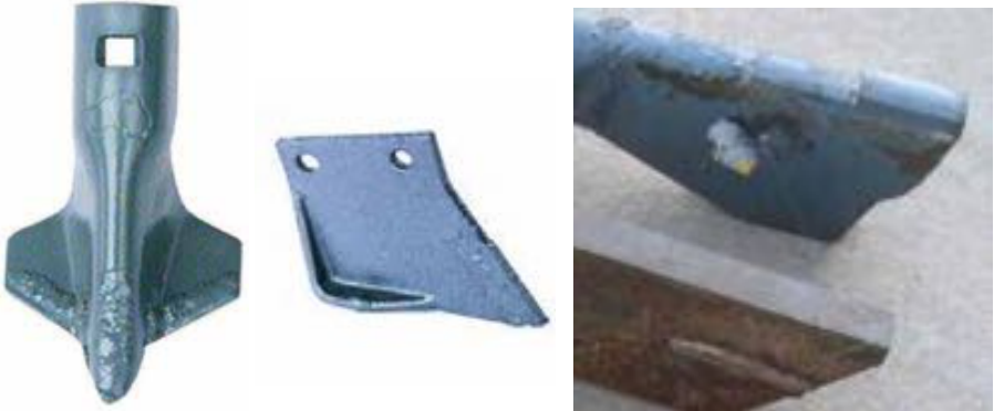
Figure 21. These Australian openers have tungsten carbide protection to enhance their durability and efficiency. The two on left have rough areas on the tip and wings where small tungsten carbide chips were welded on to the opener which is less expensive than the tile option (right) but is less durable.
