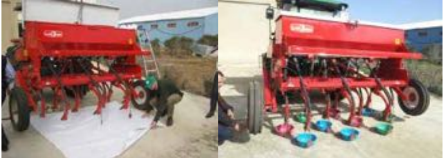
Figure 36. The output of the seeder can be collected from all tines using a large sheet of plastic to estimate the average seed or fertilizer rate (left). The uniformity of output across the seeding tines can also be measured by collecting and comparing individual outlets using small dishes labelled for each outlet (right).
