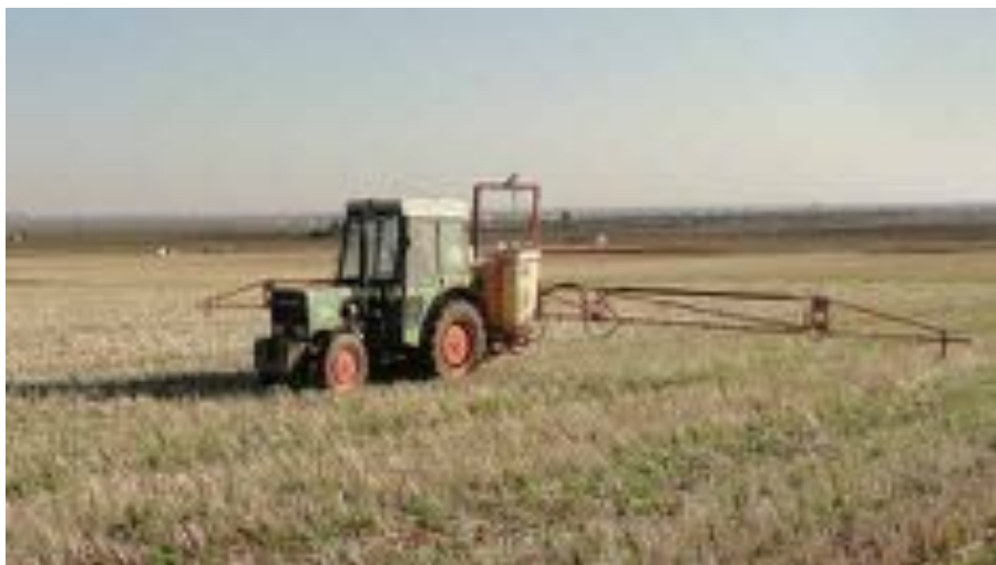
Figure 40. Most chemical sprays are applied with a boomsprayer which should be well maintained, calibrated and used in the appropriate way.
