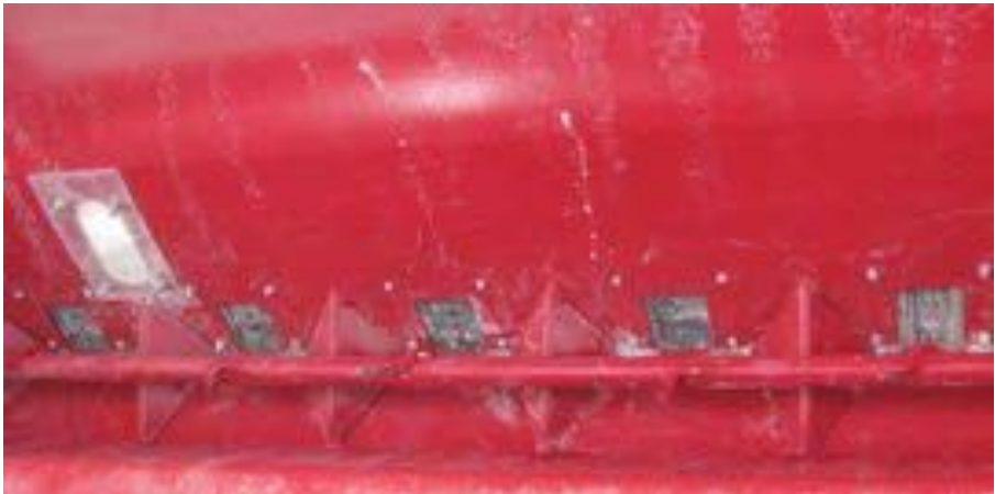
Figure 39: A clear window (left) visible from the tractor seat is a low cost solution for monitoring the seed or fertilizer levels in the hopper. Funneling inserts at the bottom of the hopper are useful to ensure each outlet does not run out of product as the level gets low.
