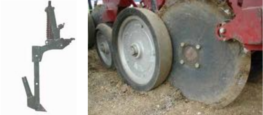
Figure 18. Examples of Australian seeding systems - a simple spring loaded tine (left), and a heavy duty single disc with gauge wheel (right).
