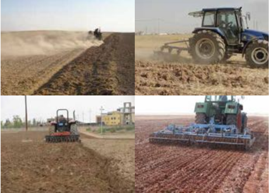
Figure 3: Moldboard and disc plowing in Syria and Iraq. Two or three tillage operations before sowing, common in the Middle East, create very high soil disturbance.
