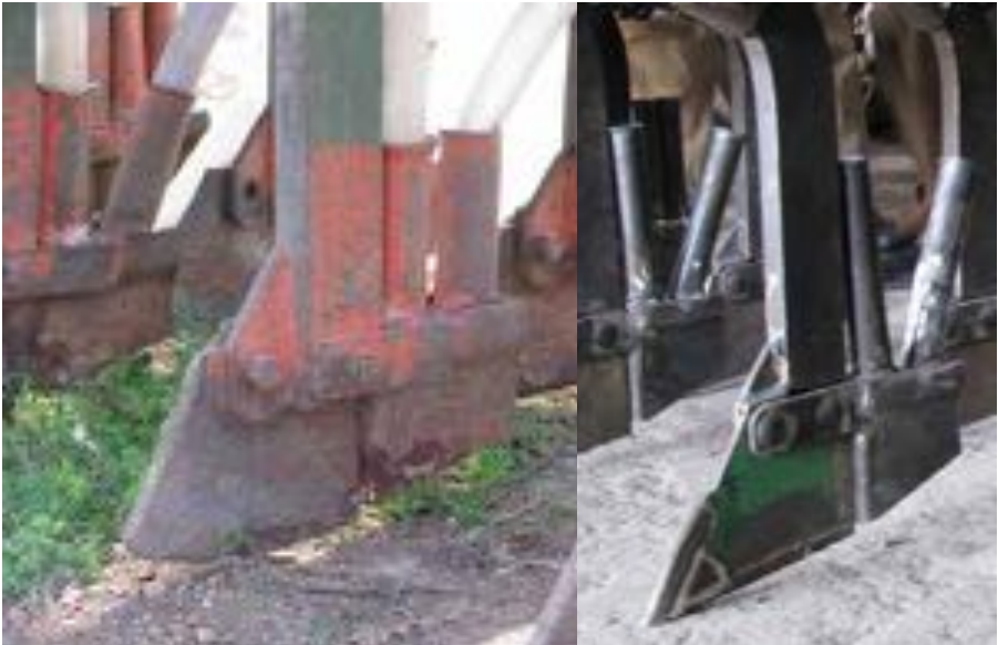
Figure 20. Badly worn knife openers (left) with a characteristic “bullnose” rounding at the leading edge will not penetrate the soil as effectively as a new opener (right).
