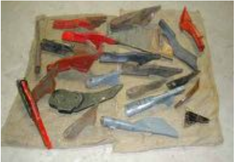
Figure 19. A selection of tine openers or narrow points with specific design features causing varying levels of soil disturbance.
