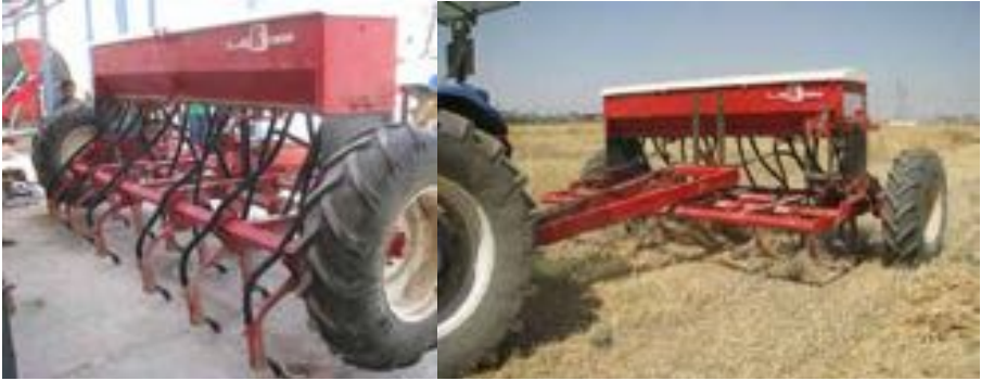
Figure 30: This conventional Rama seeder at Ainkawa Research Centre, Iraq, was converted to ZT by modifying the row spacing and tine layout, and installing narrow openers. Note the inserted black spacers to lift the seed and fertilizer boxes to create sufficient angle for the hoses. The new tine layout had a good capacity to handle crop residues (right).
