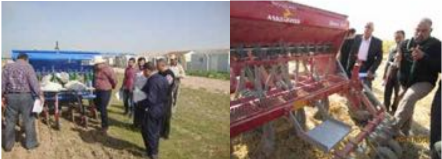
Figure 33. Field testing of the Ras Alrumh ZT seeder made in Mosul (right), and Mr. Sarmad Khalid, Directorate of Agriculture Kirkuk Iraq, discusses the ability of this Iranian ZT seeder to operate in heavy crop residues (left).
