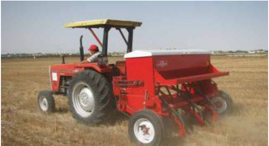
Figure 34. An example of the Rama 3 point linkage tine ZT seeder (dual hopper and 10 tines, 2.3m wide) made in Jordan in 2014 with an approximate price of US$7,000
