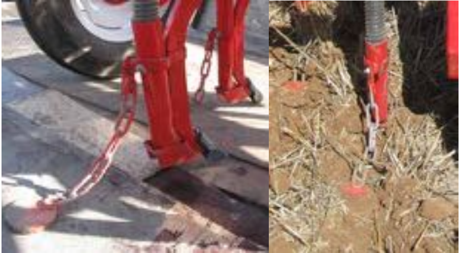
Figure 27. A 'snake chain' tine attachment with end disc can be a simple furrow closing device on a ZT seeder, particularly suited to light soil conditions.
