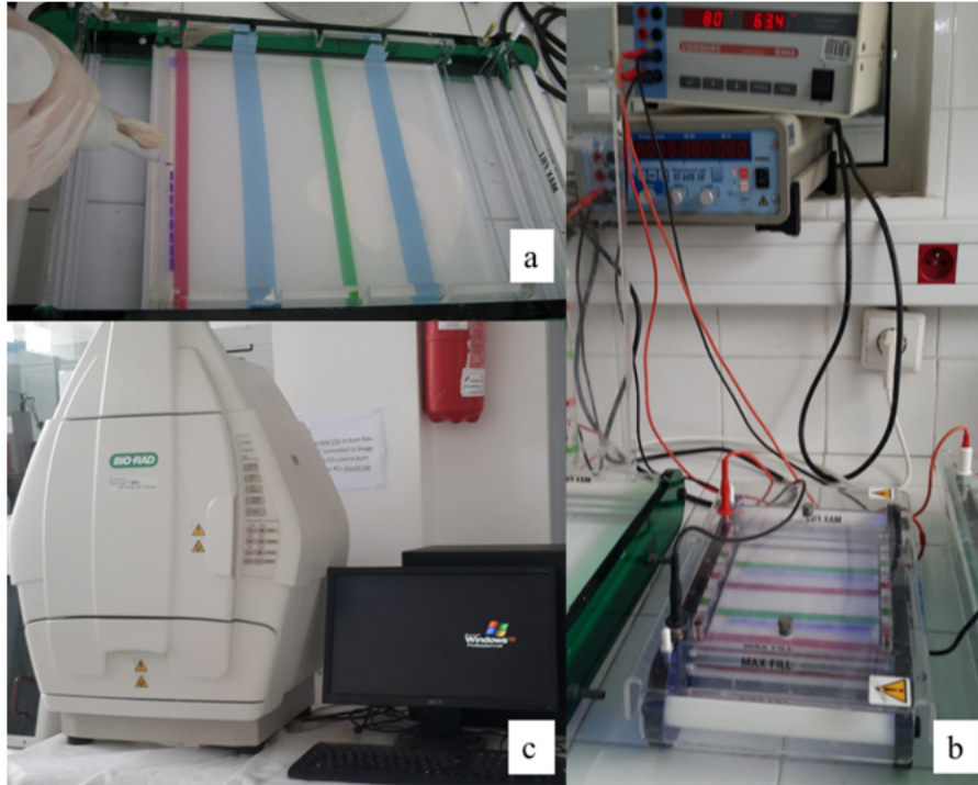
Figure 11. Deposit phase, running and visualization of 1% agarose gel
