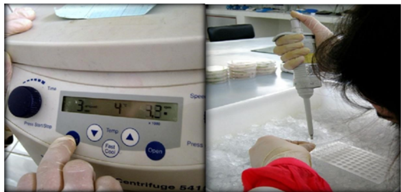
Figure 13. On the left, the master mix is being centrifuged and on the right 9 \mu L of the mix are deposited in each PCR tube
