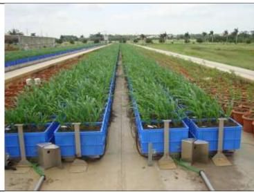
Overall view of the upgrade with load cells (left) and trays on the load cells (top) with the first dummy crop on top.
