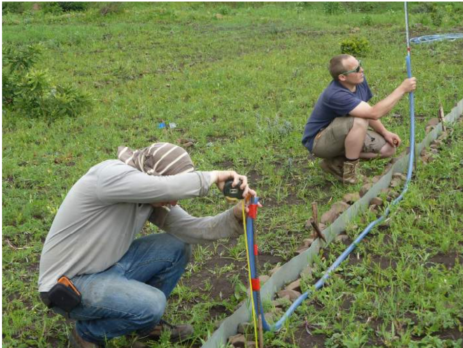
Figure 21: Surveying with a tube balance
