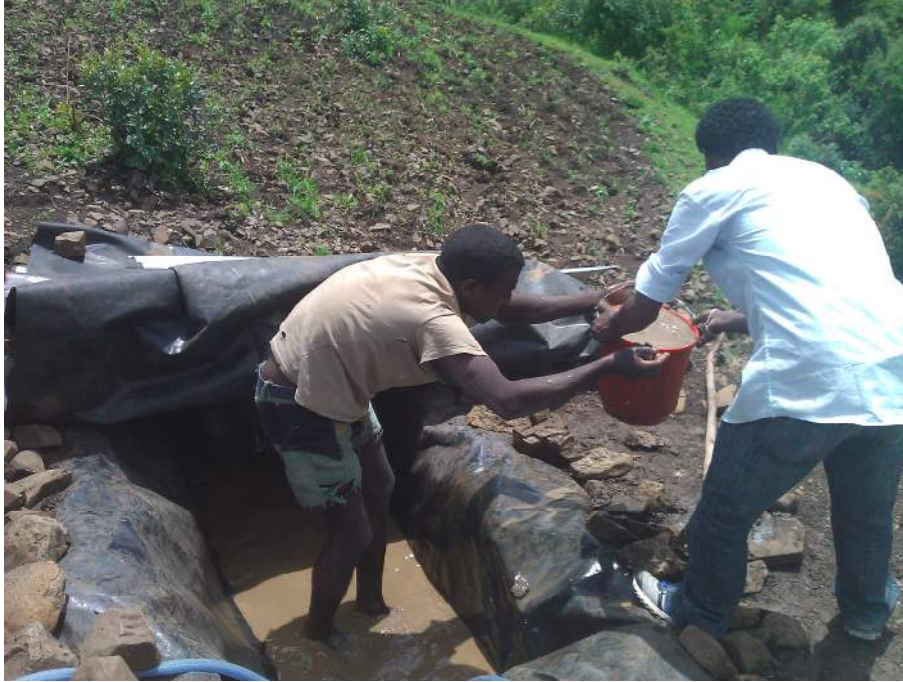
Figure 26: Estimating the water volume in a pond by emptying it with a bucket
