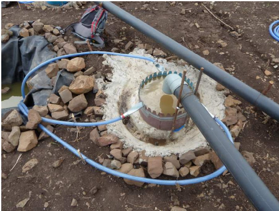
Figure 11: Sample-divider installed at the plot
