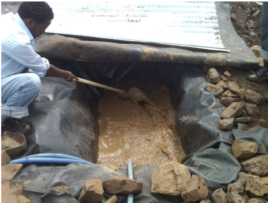
Figure 25: Stirring up the soil – water suspension in a pond before taking samples
