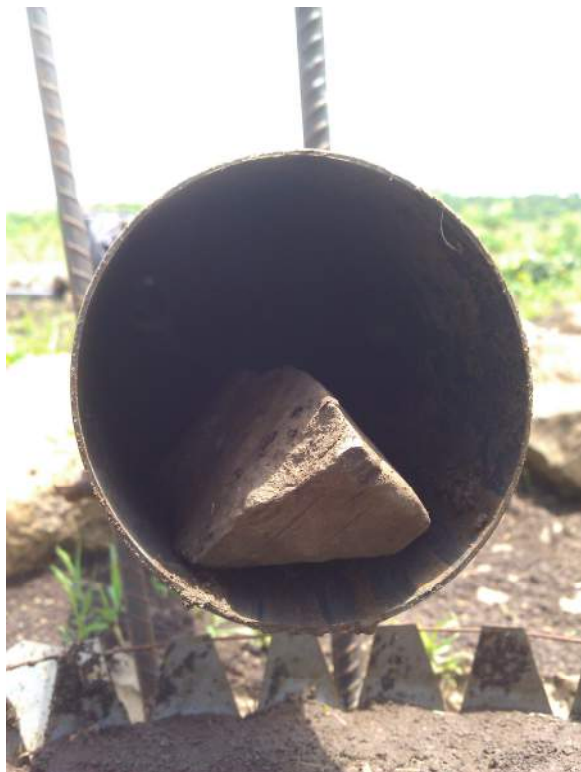
Figure 38: A big stone blocking a tube of the untreated plot
