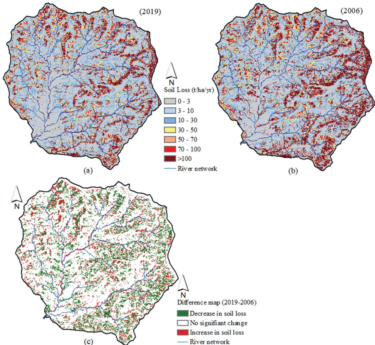
**Figure 8.** Annual soil loss estimates in 2019 (a) and 2006 (b) representing after and before watershed conservation and irrigation interventions while (c) shows difference in annual soil loss between 2019 and 2006 land use map.
