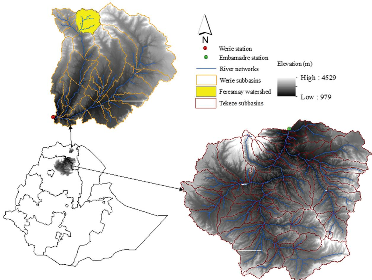
**Figure 3.** SWAT subbasin discretization for Tekeze basin and Werie watershed used for model calibration and cross-validation.
