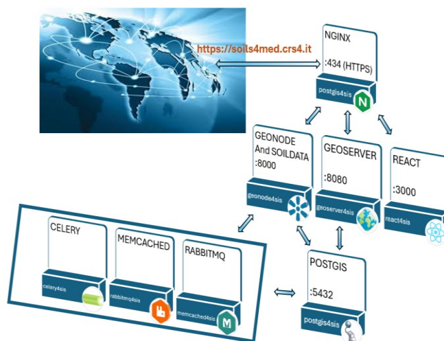
Figure 3. SIS Prototype Docker Compose Multi Container.
