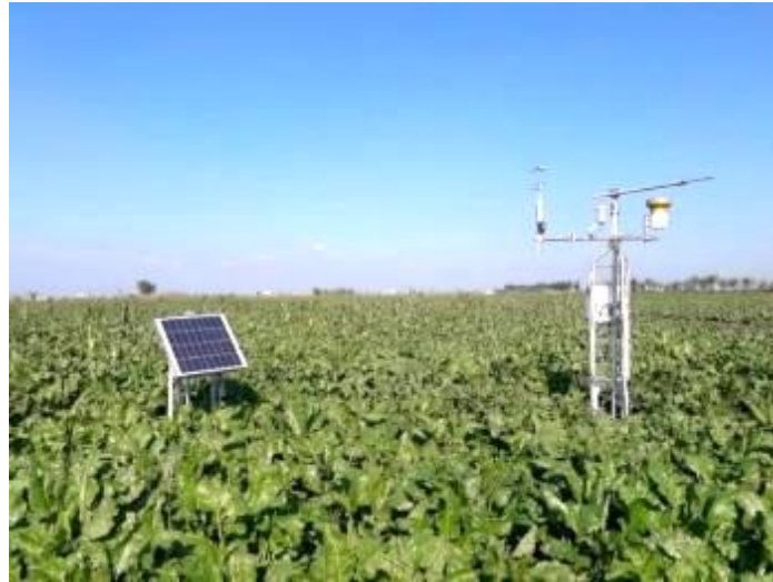
Fig. 2 – Typical example of ICARDA’s setup of eddy covariance (in this picture, the crop is sugar beet grown in old land of the Nile delta, Egypt). Courtesy: A. Swelam, personal communication.
