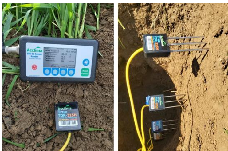
Fig. 6– Typical TDR instrument being inserted to a soil pit at a given depth. (Courtesy: Atef Swelam)
