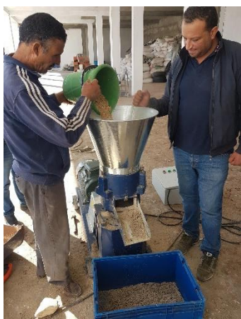
Figure 2 Feed pelletizer in use (U.Rudiger, 2023)
