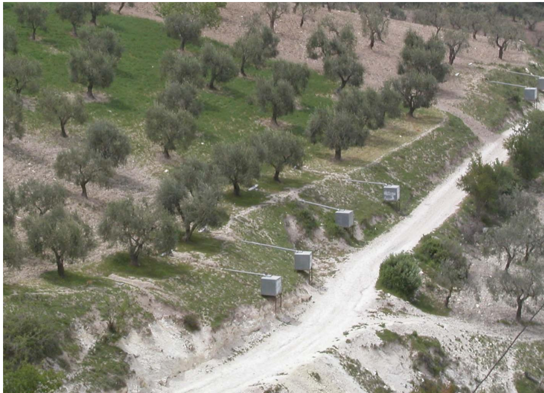
Figure 2: The Gerlach Troughs in the plots of research site No.1. Each package was measured by two Gerlach troughs.
