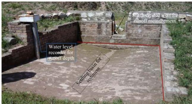
Figure 5 Experimental setup for runoff and sediment yield
