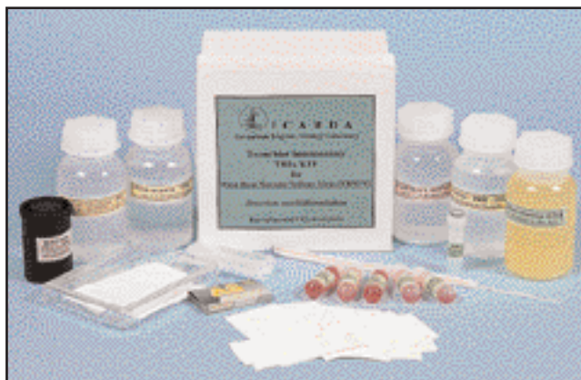
A TBIA kit for the detection of faba-bean necrotic yellows virus (FBNYV) which includes all needed reagents (buffers, sero-diagnostic reagents) as well as nitrocellulose membrane.
