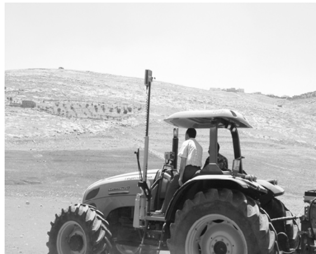
Fig. 3 Laser receiver mounted on a telescopic mast on the tractor.
