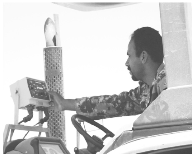
Fig. 4 Display panel mounted in front of the tractor operator.
