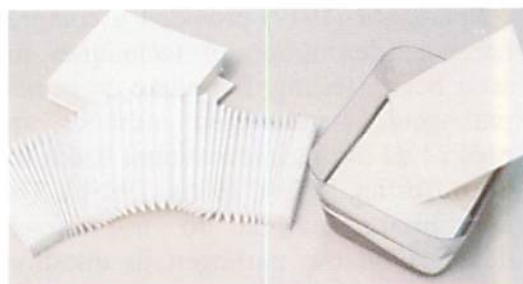
Fig. 6. Pleated filter paper strips for small seeds
