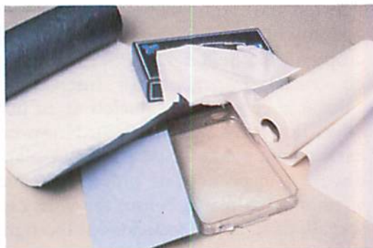
Fig. 5. Suitable media for a blotter test
