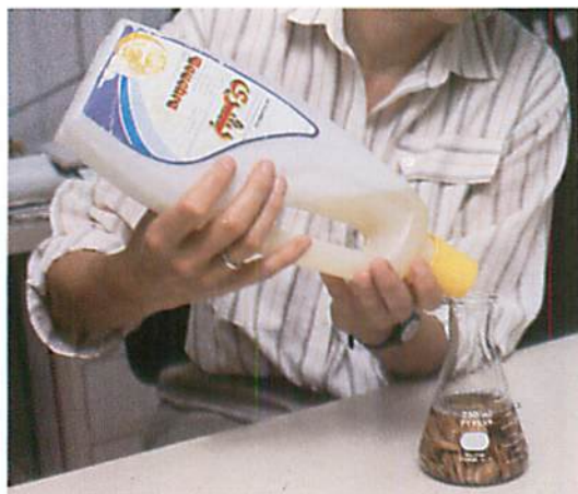
Fig. 4. Washing of seeds to remove surface-borne contamination with fungal spores. The detergent is added to reduce the surface tension
