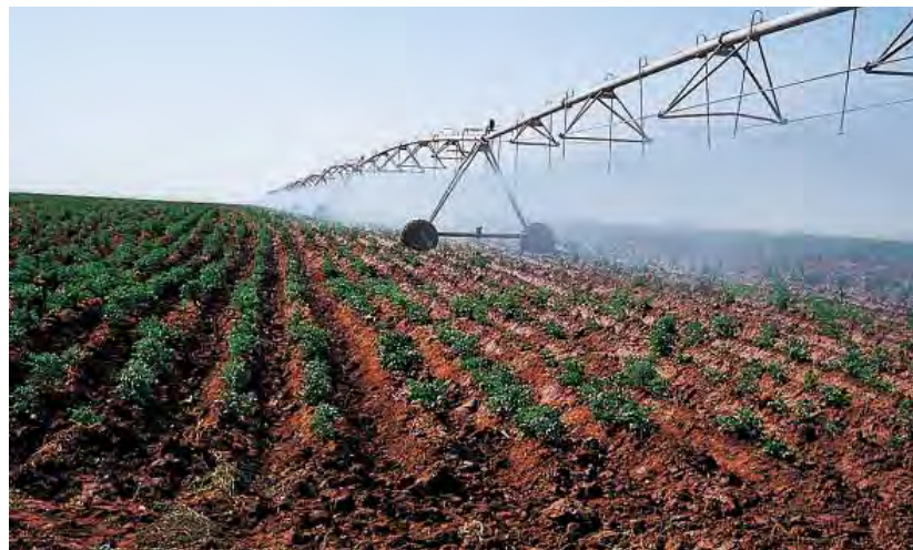
In northern Iraq, this linear-move system is used for full irrigation in summer and SI in winter.
