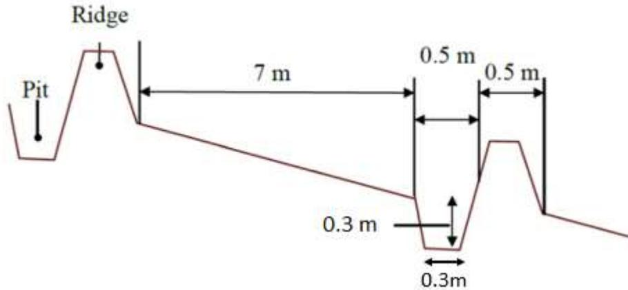
Figure 5: Schematic view of the Micro Water Harvesting structure, the Vallerani Pit (Fukai, 2019).
