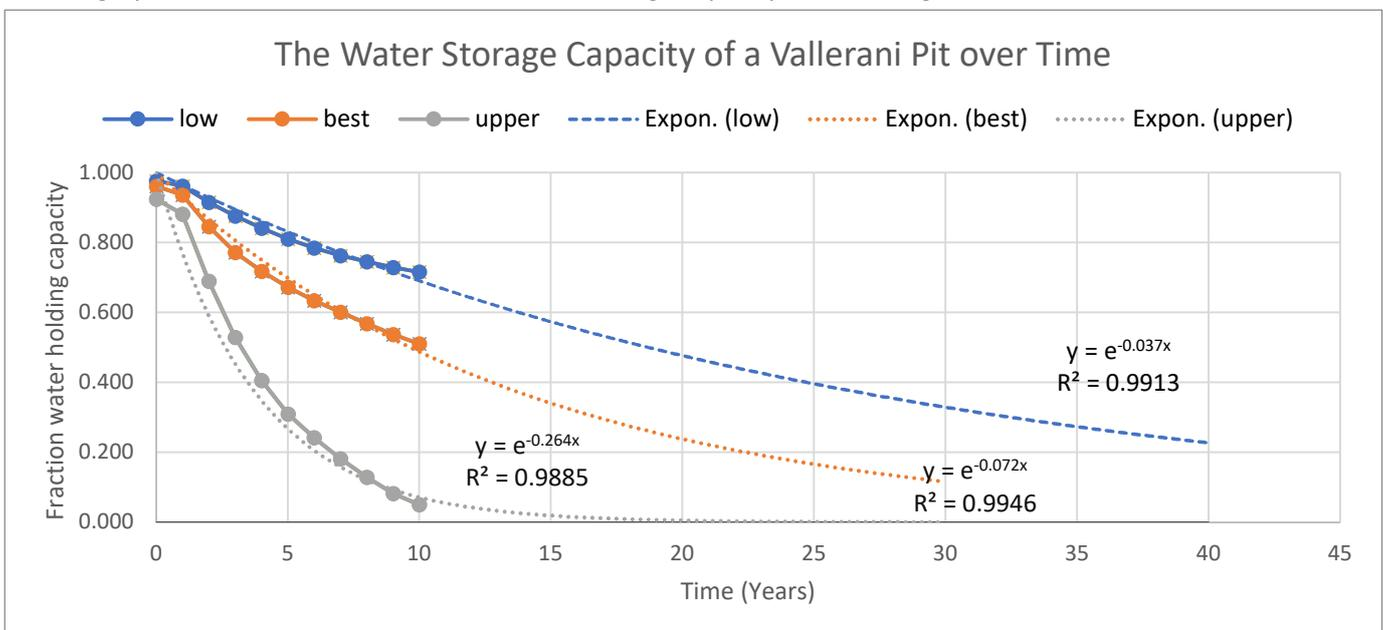
Figure 20: The Water Storage Capacity (fraction) of a Vallerani Pit over Time, with prognose.
