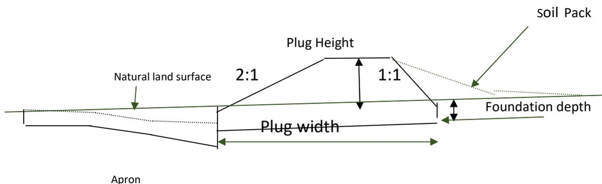
The gully plugs will be provided with an amount of soil that is resulting from the fondation to form a triangle with the structure at the upstream side this will improve the function of the gully plug in storage more water and in trapping sediments. At the other side of each structure, the slope of the side is meant to tackle the over flow of water along the drop to safely return to the gully bed level without causing additional erosion.
