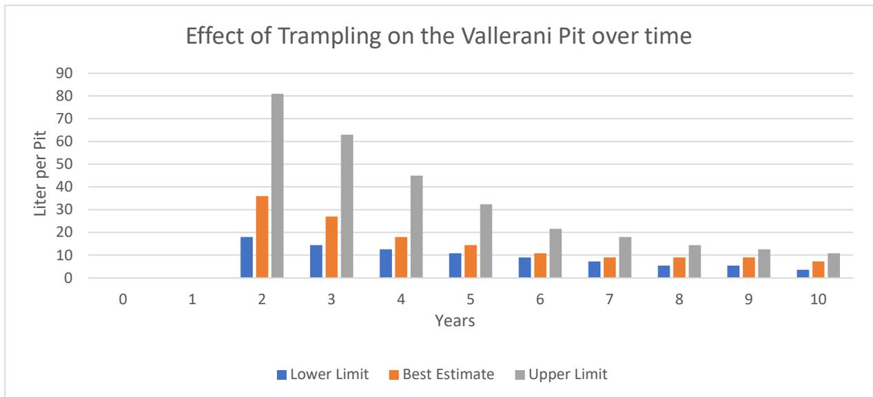
Figure 17: Effect of Trampling by livestock on the Vallerani Pit with respect to Time
