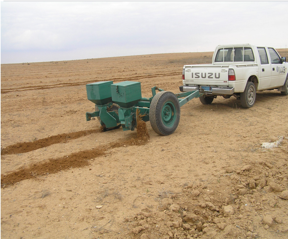
Direct seeding using pitting machine, Aleppo – Syria
