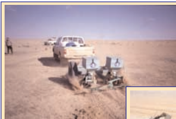
For slightly deeper, loamy soils the ICARDA team, led by range specialist Dr Gus Gintzburger built a pitting machine (above and right) which scoops a shallow pit in the soil into which the seed of local desirable species is dropped, then lightly covered by the following tines.
