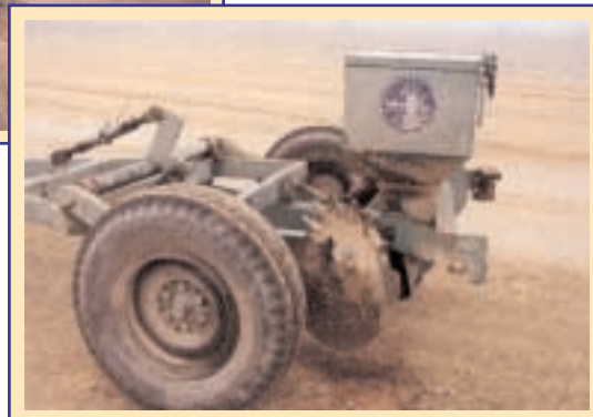
For slightly deeper, loamy soils the ICARDA team, led by range specialist Dr Gus Gintzburger built a pitting machine (above and right) which scoops a shallow pit in the soil into which the seed of local desirable species is dropped, then lightly covered by the following tines.
