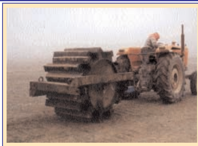
Converted in the ICARDA workshop from a 3t roller, the Land Imprinter is solidly built, low-tech and can be pulled easily across the steppe with a small tractor.
