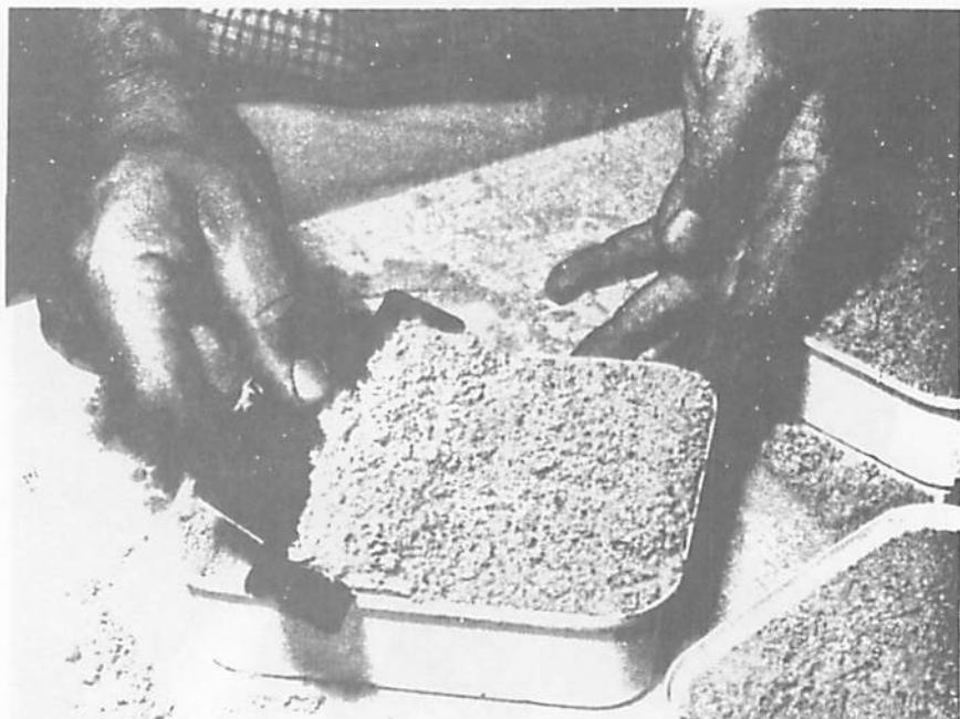
Fig. 9. The surplus of sand is removed with the long side of the scraper.
