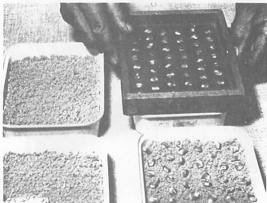
Fig. 6. The counting board is placed on top of the seed bed and the lower plate is pulled to release the seeds.
