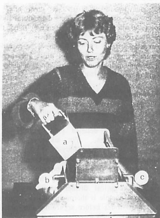
Fig. 1. Soil divider. The first of a series of halvings is shown. The three pouring pans are labelled (a), (b), and (c).
