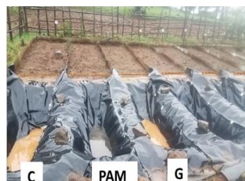
Experiment on the effectiveness of soil amendments C: Control; PAM: Polyacrylamide, G: Gypsum
