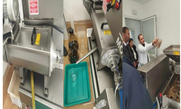
Step 4. Oil is separated from the solids
