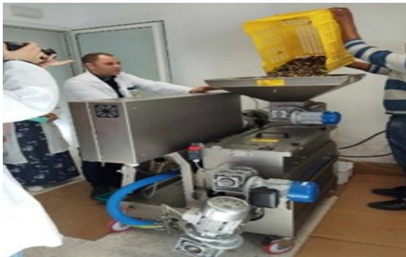
Step 1. Putting the olives into the press
