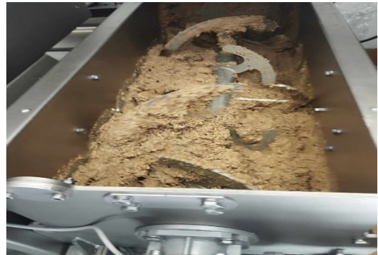
Step 2: Olives are crushed into a paste
