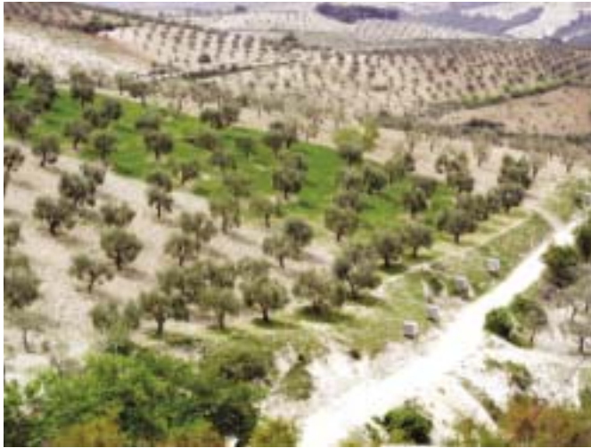
Plate 1 The layout of the Gerlach troughs in the plots of the research site. Two Gerlach troughs, consisting of 2 m of collecting gutters, were dug into the soil at the bottom of slope position in each of the manure, vetch, and farmer-practice treatments
