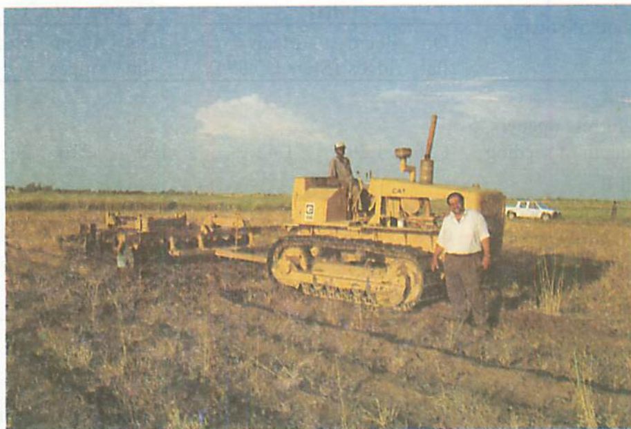
Fig. 5. Seed drill for sowing wheat in rows.
