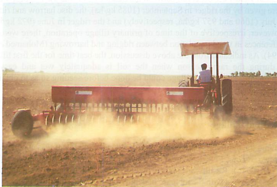
Fig. 2. Wide level disc, combining tillage and seed drilling.
