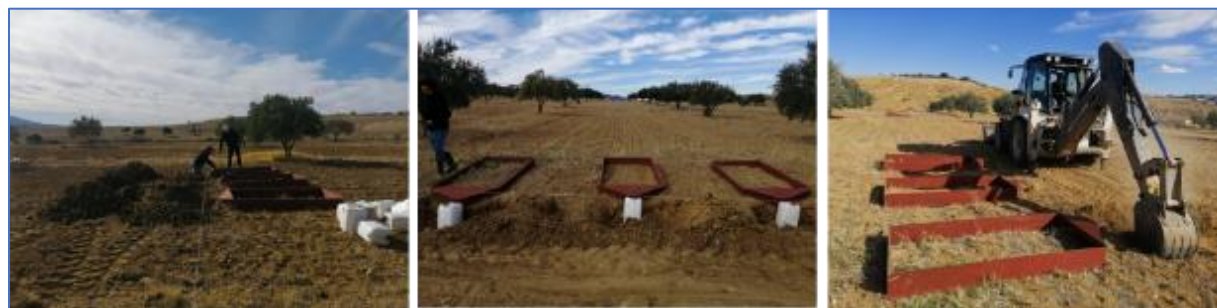
Photo 2. Installation of the Wischmeier protocol for soil erosion measurement in Kairouan (Oued Elgsab).
