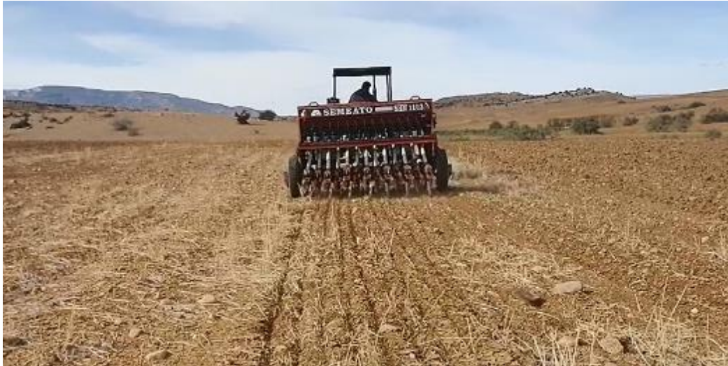
Photo 8. Sowing of forage mixtures in pure stand in no-tillage plot using no-till seeder
