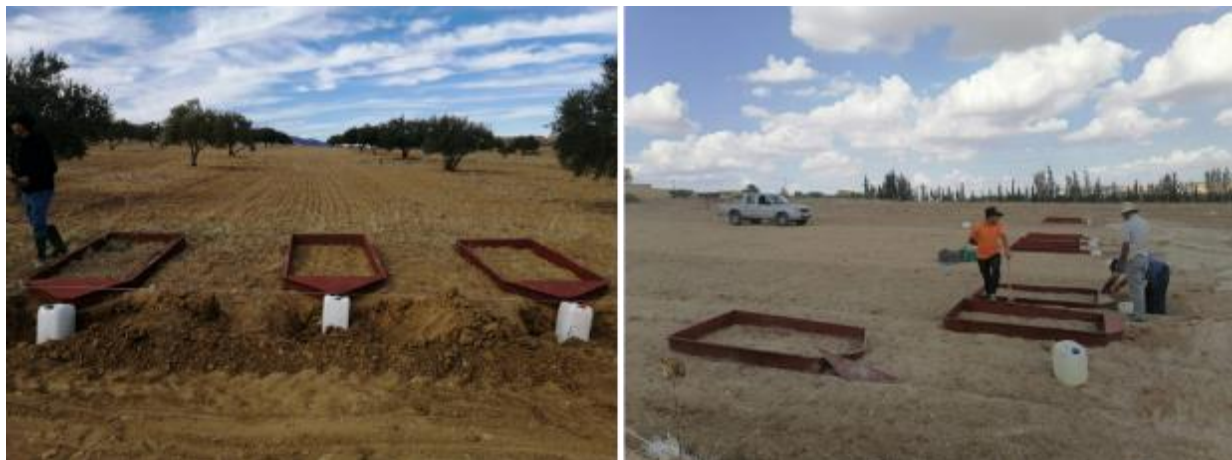
Photo 1. Installation of the Wischmeier protocol for soil erosion measurement in Siliana and Kairouan sites
