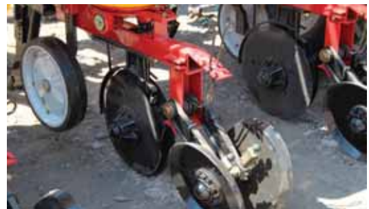
Photo 2: Disc opener, gauge wheel, double disc closing wheels
