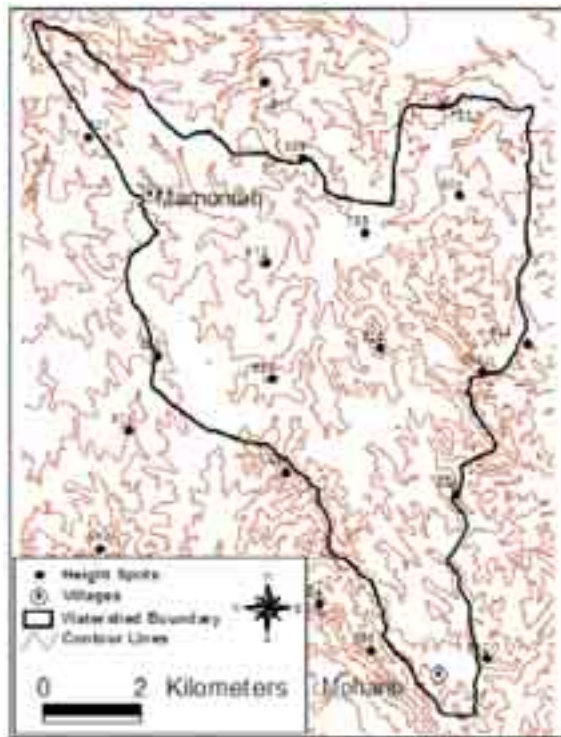
Source: Royal Jordanian Geographic Center (1:50,000 topographic maps) Figure 32: Contour lines and spot heights for watershed no. 104.
