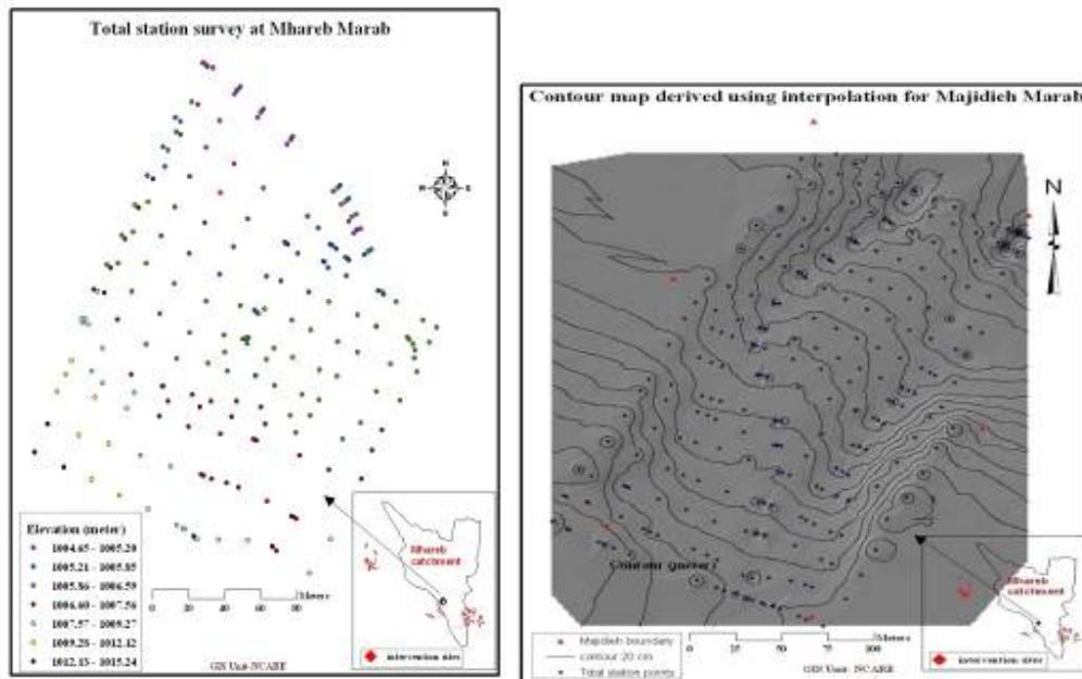
Figure 5: Total station survey and converting to (X, Y, Z) at Marab to contour map
