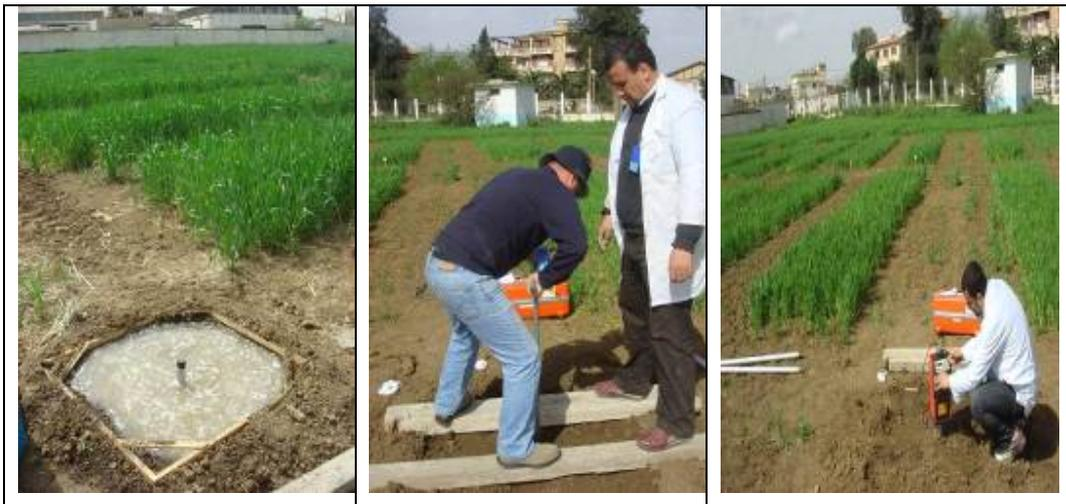
**Photo 1: Neutron probe calibration and field capacity test**
