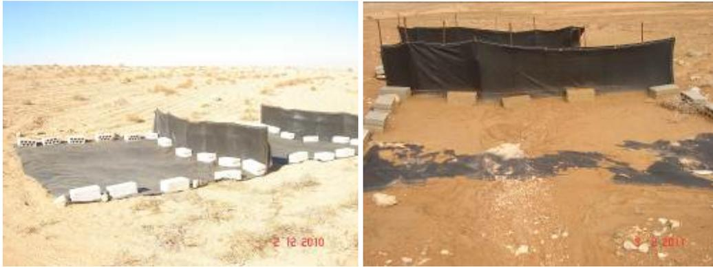
**Figure 2: Geotextile construction for sediment data collection**
