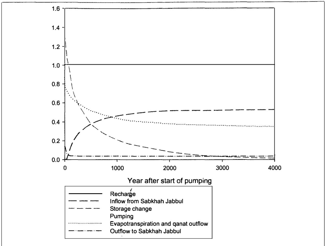
Figure 4. Example of simulated changes in flow volumes over time as a response to current pumping rates.
