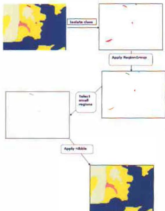
Figure 82. Steps for removal of noisy pixels
