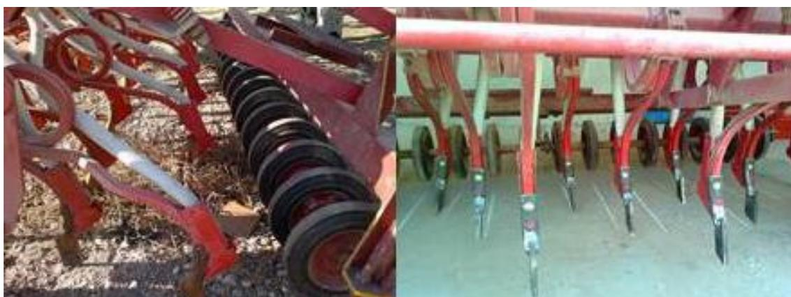
**Fig (3): Gaspardo seeder after modification to ZT seeder and adding press wheels.**
