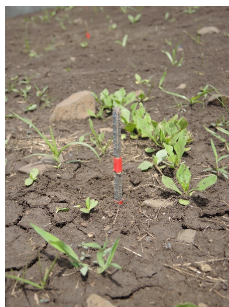
Figure 4-16: Single erosion pin (photo: S. Wakolbinger)
