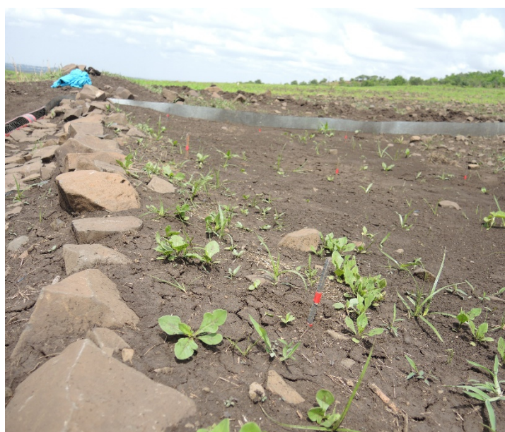
Figure 4-15: Erosion pin arrangement in the accumulation zone (photo: S. Wakolbinger)
