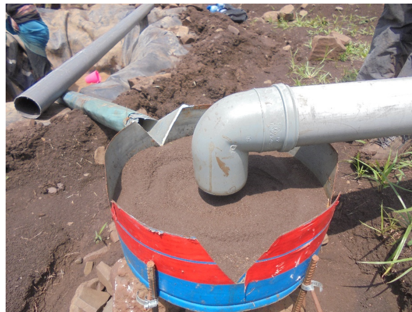
Figure A.1-6.2: Sedimented sample divider (photo: E.Obereder)
