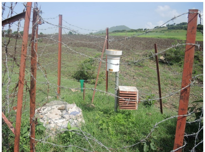
Figure 4-12: Tipping bucket ombrometer (photo: N. Demelash)
