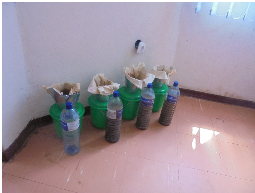
Figure 4-24: Filtering system including plastic buckets, metal cones and textile filters (photo: S. Wakolbinger)
