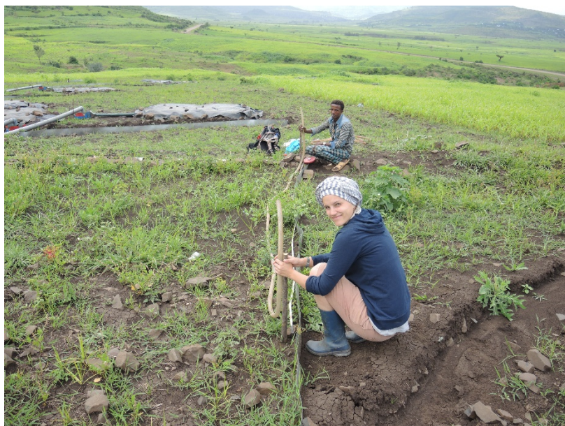
Figure 4-13: Inclination assessment with the tube water level (photo: E. Obereder)
