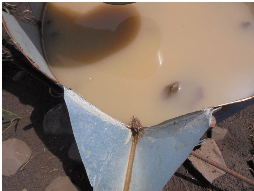
Figure A.1-6.1: Blocked sample divider cut (photo: E.Obereder)
