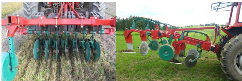
Figure 17. Left: vertical and right: horizontal root cutter prototypes by Kvaerneland company
