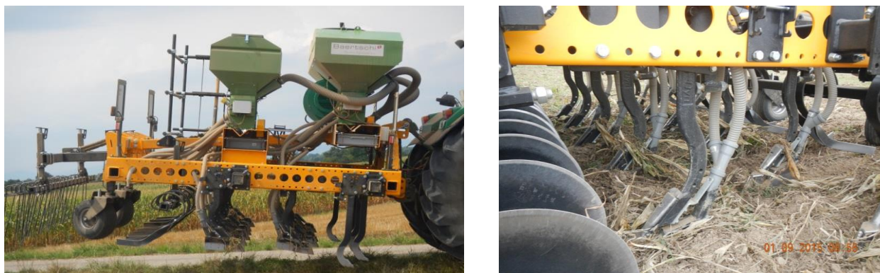
Figure 12. Left: Machine equipped with no-till chisels/furrow openers. Front row has narrow cultivator tines. The bounce plates for broadcasting seeds are placed in between the support wheels at the rear, just before the harrow. Right: Machine with discs running in front of furrow openers.
