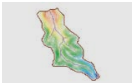
Topographical and hydrological layers of the Chaluk water harvesting site, one of several identified in the HSAD pilot. The site identification method developed by ICARDA combines ground-level assessment of slope and soil, GIS imaging and socio-economic information about the proximity of the local population. A national plan targets the creation of some 80 hill lakes to provide stable irrigation for crops produced in the driest seasons – a positive impact for thousands of rural inhabitants.
